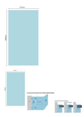
This panel can be used as a return panel when installing a corner shower or a fixed panel when installing a single panel screen.
