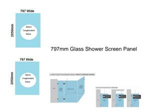
This panel can be used as a return panel when installing a corner shower or a fixed panel when installing a single panel screen.
