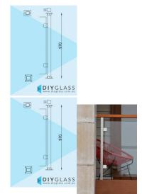
50x50 Square Glass Clamp End Post for Timber Rail •Position: End •Use: Glass Balustrade •Material: 50x50 Satin Finish Stainless Steel •Height: 970mm •Grade: 316 Marine Grade Stainless •Base: 4 Hole Square Flange •Top: 2 Hole Rectangle Flange •Glass: Install with 850mm Glass Panels •Handrail: Install with Timber Handrail
