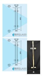
2" Round Glass Clamp Centre Post for Timber Rail •Position: Centre •Use: Glass Balustrade •Material: 2" Mirror Finish Tube •Height: 970mm •Grade: 316 Marine Grade Stainless •Base: 3 Hole Round Flange •Top: 2 Hole Oblong Flange •Glass: Install with 850mm Glass Panels •Handrail: Install with Timber Handrail
