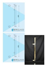
2" Round Glass Clamp End Post for Timber Rail •Position: End •Use: Glass Balustrade •Material: 2" Mirror Finish Tube •Height: 970mm •Grade: 316 Marine Grade Stainless •Base: 3 Hole Round Flange •Top: 2 Hole Oblong Flange •Glass: Install with 850mm Glass Panels •Handrail: Install with Timber Handrail
