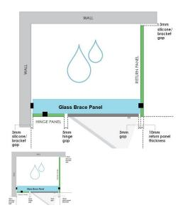
Glass Brace panel used to Connect the hinge panel to a return panel above the door.
