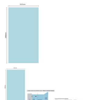
This panel can be used as a return panel when installing a corner shower or a fixed panel when installing a single panel screen.
