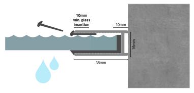
**TRADE TIP:** Temporarily hold the L-shape rubber in place with tape to assist with glazing the 10mm glass panel.
