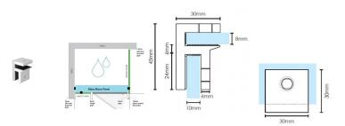
Used to stiffen and brace a return or hinge panel by fixing a brace panel along the top and tying them together.
