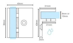
Used to fix Hinge and Return/Fixed panels to the wall in a shower screen.
