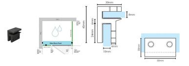
Used to stiffen and brace a return or hinge panel by fixing a brace panel along the top and tying them together.
