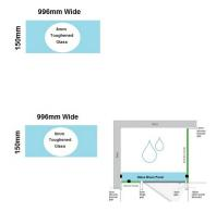
Glass Brace panel used to Connect the hinge panel to a return panel about the door. •Width: 996mm •Depth: 150mm •Thickness: 8mm •Weight: 3.0kg •Use With Hinge Panel: 379mm Requires 2 x Glass Brace Brackets and 1 x Wall Bracket for Installation.
