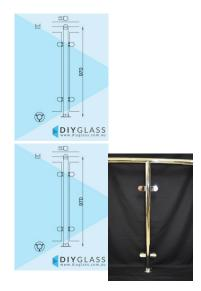
2" Round Glass Clamp Centre Post for Stainless Top Rail •Position: Centre •Use: Glass Balustrade •Material: 2" Mirror Finish Tube •Height: 970mm •Grade: 316 Marine Grade Stainless •Base: 4 Hole Square Flange •Top: Perpendicular Joiner •Glass: Install with 850mm Glass Panels •Handrail: Install with 2 Inch Round Stainless Top Rail The perpendicular joiner is Tek screwed to the underside of the rail then glued and riveted into the top of the post.
