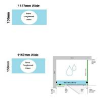
Glass Brace panel used to Connect the hinge panel to a return panel about the door. •Width: 1157mm •Depth: 150mm •Thickness: 8mm •Weight: 3.6kg •Use With Hinge Panel: 540mm Requires 2 x Glass Brace Brackets and 1 x Wall Bracket for Installation.
